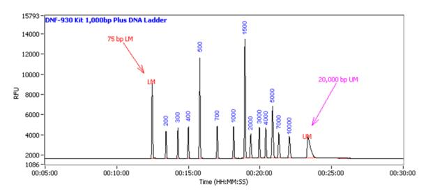
Representative 1,000 bp Plus DNA Ladder result injected with 75 bp lower marker and 20,000 bp upper marker, using the ZAG system with the ZAG-130-5000 reagent kit. Method: **ZAG130FC33** (short array).
